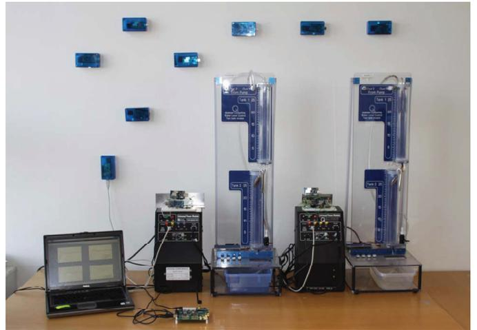
Fig. 2. Setup for the coupled water tank systems and the WSN.
